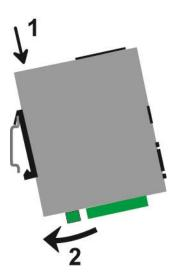
Removing the unit from the DIN rail
