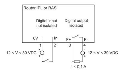
To check that the input and the output are correctly wired, select
